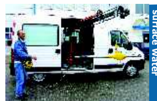
vehicle with crane and current meter
