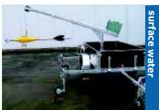
SEWII with mobile jib and current meter
